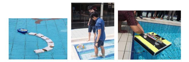
Figure 9. Some of the student projects in Engineering Design (a) Snake robot for filtering oil from ocean surface (b) amphibian vehicle (c) a sensor station collecting several sensor readings and transmitting to a computer wirelessly.
