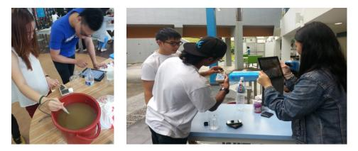
Figure 8. (left) Measuring the pH and turbidity of dirty water, (right) measuring the pH and turbidity of filtered water
