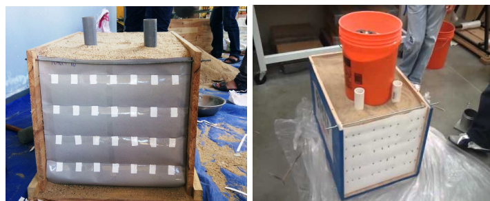
Figure 2. Test of retaining wall models made from carton paper
