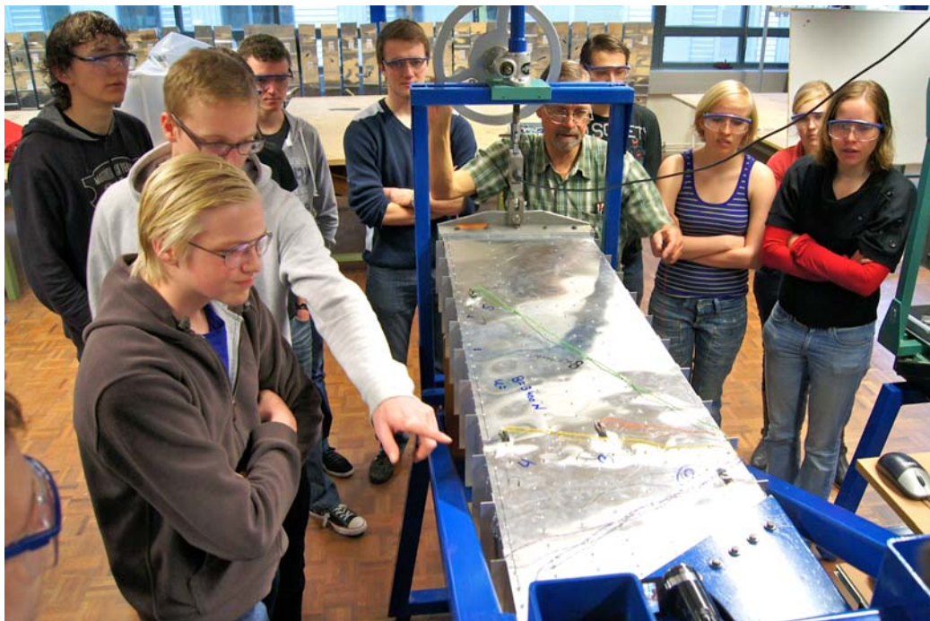
Figure 5 Testing the light-weight structural box of a wing, designed and manufactured in the second design project
